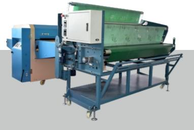
UNIX is pleased to introduce a revolutionary technology of printing rhinestone without any film or paper, directly on the fabric. It comes with two units, the first unit puts the rhinestones on the fabric, and the second unit does fusing to fix the rhinestone. So, ultimately, this technology eliminates the one complete step in this process •
